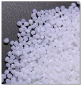
Polyester is dried further and then extruded into pellet.
