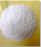
Cellulose is dried into a powder.
